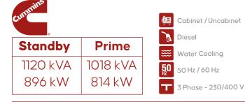
**Standby Power (ESP):** In case of failure of reliable mains supply.variable electricity is used to power the load. ESP complies with ISO8528. Overloading is not allowed.
