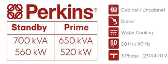
**Standby Power (ESP):** In case of failure of reliable mains supply.variable electricity is used to power the load. ESP complies with ISO8528. Overloading is not allowed.
