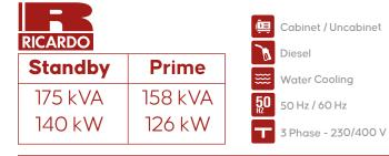
Standby Power (ESP): I h case of failure of reliable mains supply.variable electricity is used to power the load. ESP complies with ISO8528. Overloading is not allowed.
