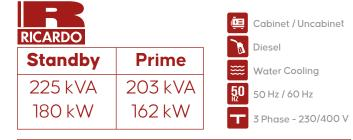
**Standby Power (ESP):** In case of failure of reliable mains supply.variable electricity is used to power the load. ESP complies with ISO8528. Overloading is not allowed.
